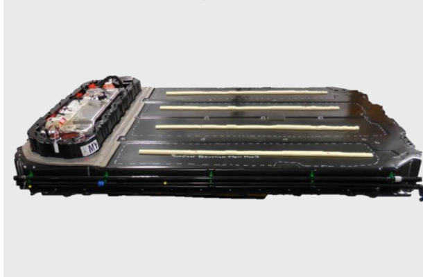
Tesla Model Y 배터리팩
