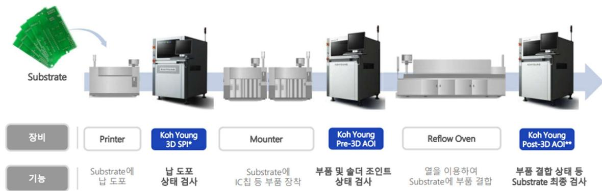
주: SPI(Solder Paste Inspection, 납도포 검사기), AOI(Automated Optical Inspection, 자동광학검사)
