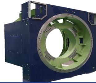
**Generator Stator Frame**
