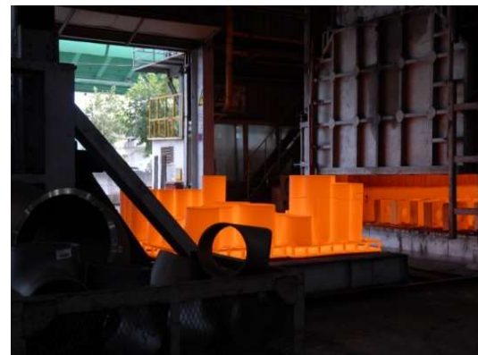
Solution Heat Treatment Furnace
