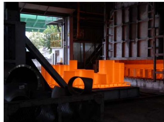
Solution Heat Treatment Furnace
