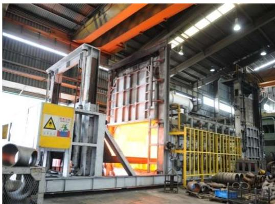
Heat Treatment Furnace For Fitting
