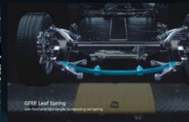
Multi Functional GFRP⁴ Leaf Spring
