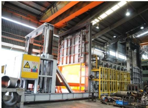
Heat Treatment Furnace For Fitting
