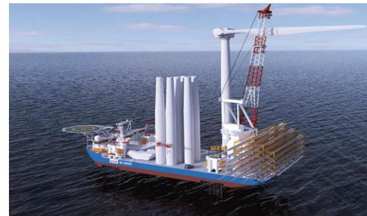
해상풍력설치선 (Wind Turbine Installation Vessel)
