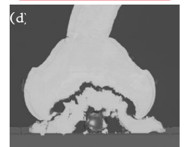
③ Wire Crack
