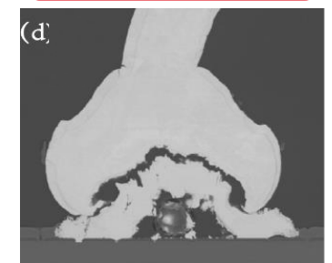
③ Wire Crack
