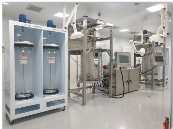
Peptide synthesis Reactor (반응기 SUS, 300ℓ X 10대)
