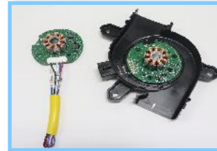
Blower Motor Driver
