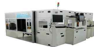
Bumped wafer 2D/3D Inspection System
