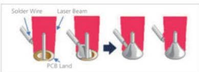
Laser Soldering Process (With Solder Wire)
